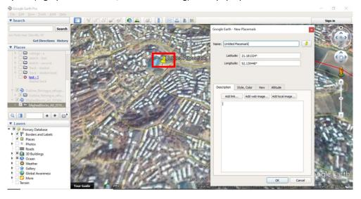
Prefer to use decimal degree format for collecting point. So before taking a point change the setting in decimal degrees from tool to Show Lat/Long in Decimal Degree.
